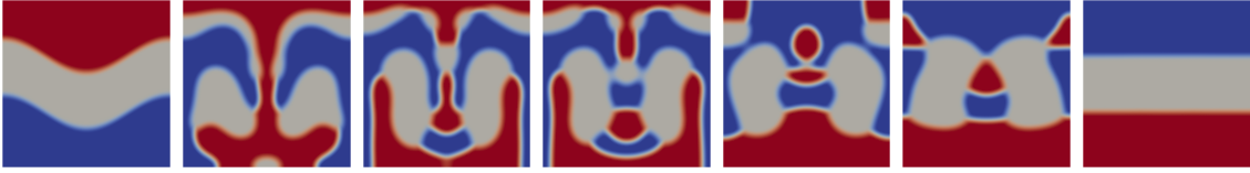
FIGURE 4. Evolution of the density of a three component mixture at t = 0, 4, 5.4, 5.8, 9, 11.6 (from left to right).
