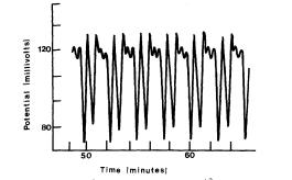
Recording from bromide ion electrode; T=25  $^{\circ}$  C; flow rate = 3.99 ml/min; Ce<sup>+3</sup> catalyst [Hudson, Hart, Marinko '79]
