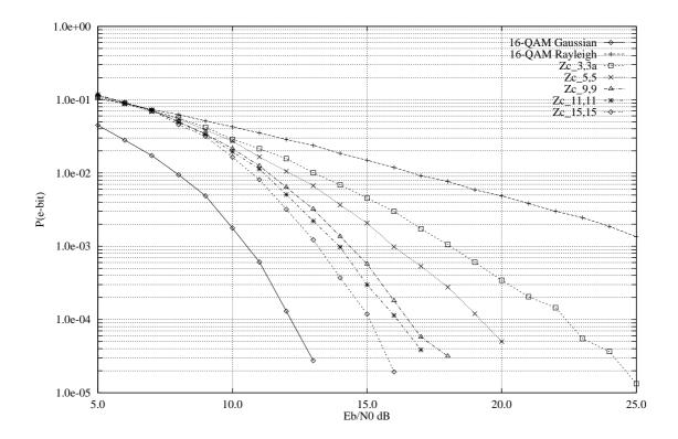
Fig. 9. Bit error rates for the family of  $Z_{n,n}$  constellations from  $\mathbf{Q}(2\cos(2\pi/N))$   $(\eta=4)$
