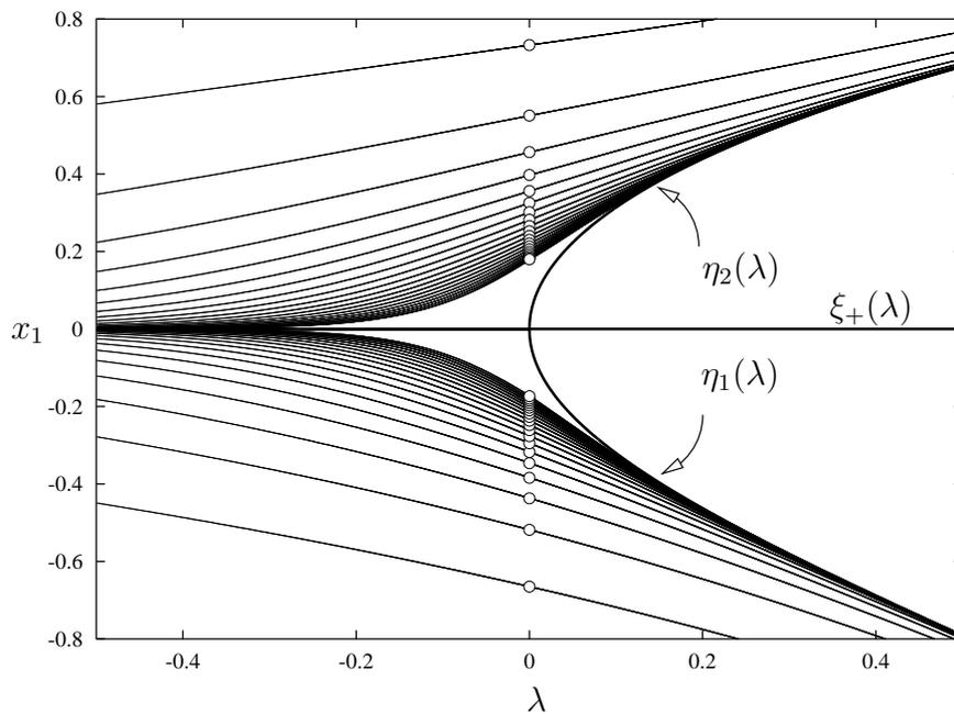
Figure 12: A neighborhood of the flip bifurcation at  $\lambda = 0$ , projected onto the  $(\lambda, x_1)$ -plane. Additionally, the fixed points and two-periodic orbits are displayed.
