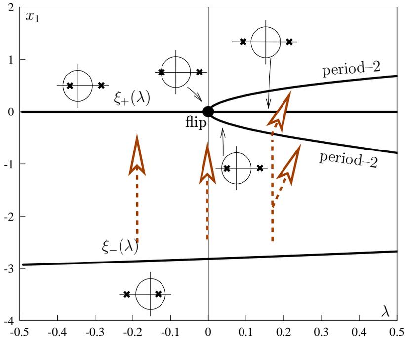
Figure 10: *Bifurcation diagram of fixed points of  $f$ , projected onto the  $(\lambda, x_1)$ -plane. The big arrows mark the fixed points and two-periodic orbits, connected during the numerical continuation.*
