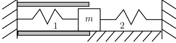
**Figure 5.1** A mass controlled by two springs.
