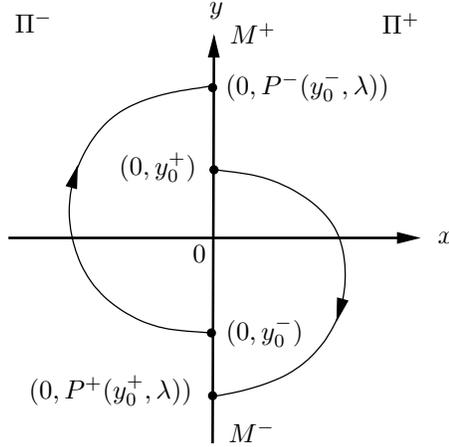
**Figure 3.1** Illustrations of the Poincaré map for each linear subsystem of (3.1).
