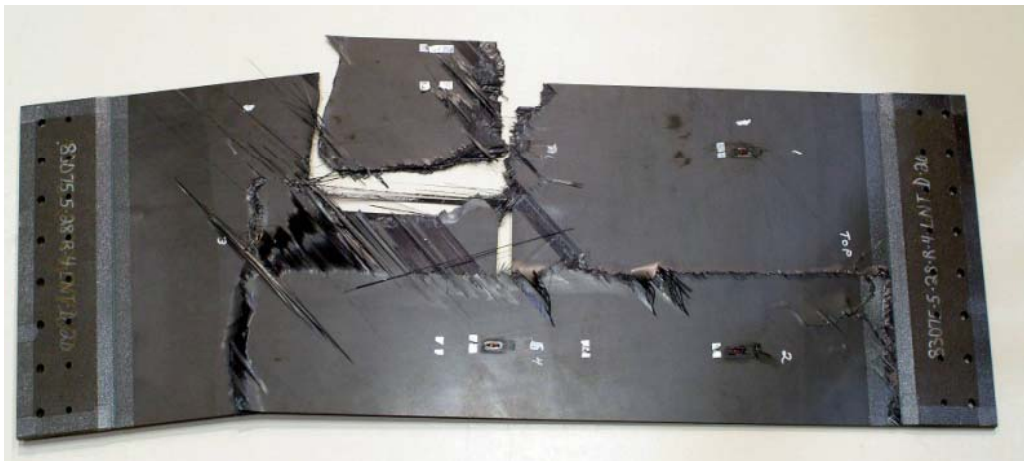
Typical crack growth in notched laminate (photo courtesy Boeing)
