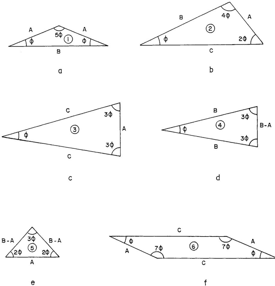
Fig. 1. Fundamental shapes of our tiling ( $A = 1.000$ ,  $B = 1.802$ ,  $C = 2.247$ , and  $\Phi = \pi/7$ )
