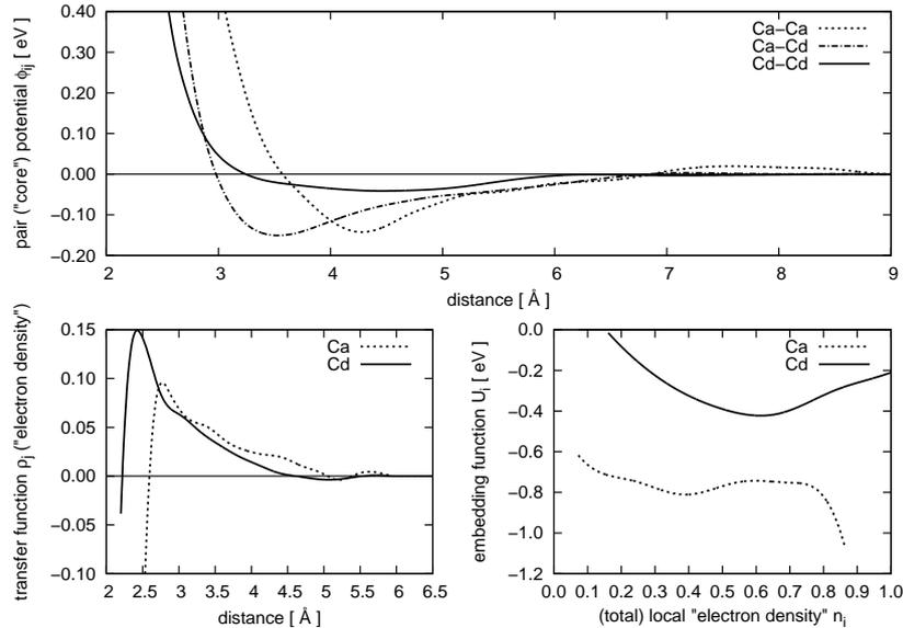
Figure 1. Potential functions of the Ca-Cd EAM potential.
