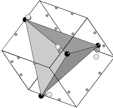
Figure 2. Ideal tetrahedron, compared to Gómez-Lidin tetrahedron. The corners of the Gómez-Lidin tetrahedron (large medium gray dots) relax to new positions (black dots). The light gray dots are corners of other relaxed tetrahedra, so that the total number of possible tetrahedron corners is doubled. Shown are also the other Gómez-Lidin tetrahedron corners as smaller medium gray dots. The cube is drawn as a guide to the eye.
