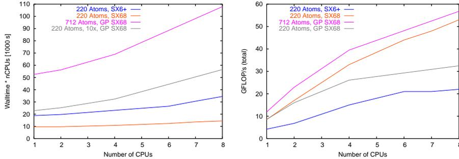
**Fig. 1.** Scaling of VASP for different systems on the SX8 (with SX6 executables) and the SX6+. Shown are total CPU times (left) and absolute gigaflop rates (right). The timings of the 220 atom system ( $\Gamma$ -point only version) on the SX8 have been multiplied by 10.
