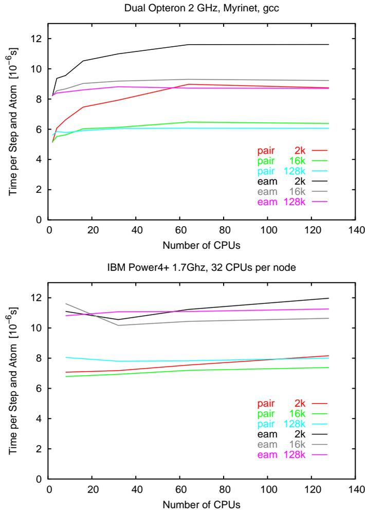
**Fig. 4.** Scaling of IMD on the Opteron (top) and IBM Regatta (bottom) systems.
