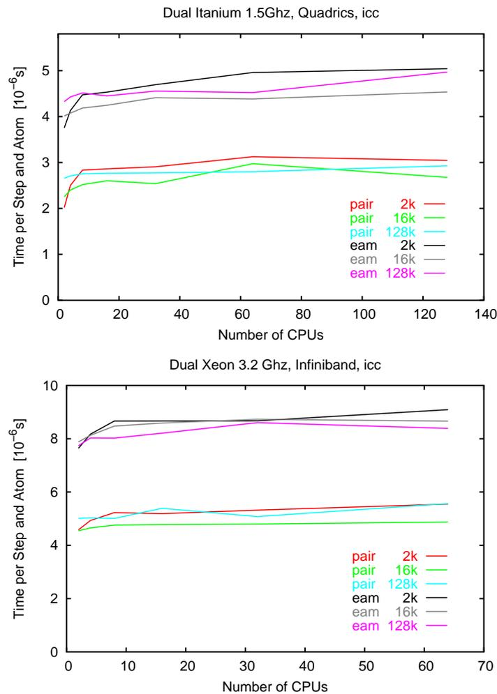
Fig. 3. Scaling of IMD on the Itanium (top) and Xeon (bottom) systems.
