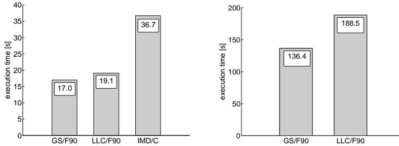
**Fig. 9.** Execution times of the different algorithms on the NEC SX8, for FCC crystals with 16k atoms (left) and 131k atoms (right).
