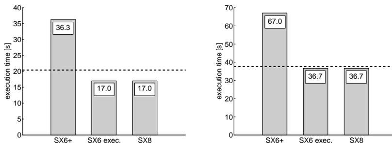
**Fig. 10.** Execution times on SX6+ and SX8 for an FCC crystal with 16k atoms using Grid Search (left) and IMD (right).
