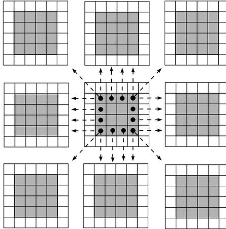
**Fig. 2.** Decomposition of the sample into blocks and cells. Each CPU deals with one block of cells. The white buffer cells contain copies of cells on neighbor CPUs, so that forces can be computed locally.
