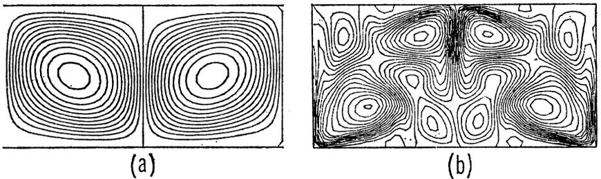
Fig. 2. (a) Conventional analysis could yield the steady-state streamline pattern in a Bénard problem for  $R = 3 \times 10^4$ . (b) Only the computer could reveal the details of the unsteady flow at  $R = 3 \times 10^6$ , of which this is typical streamline pattern.
