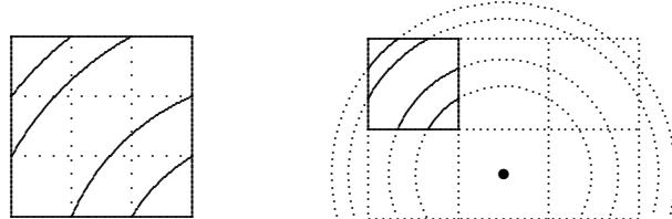
Let us return to the first “impossible dovetail” problem considered at the beginning of this section, but use the construction methods just discussed. We see that the previous picture in the middle yields a solution of the starting problem, now using circular dovetails instead of straight ones.
