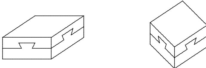
Can such a double-dovetail be realized? To be precise, it should be made from two pieces of wood, without any excavation, and made without any trick (such as using moistening and damping, or using pressure) - thus we are looking for a solution with a genuine geometrical construction.
