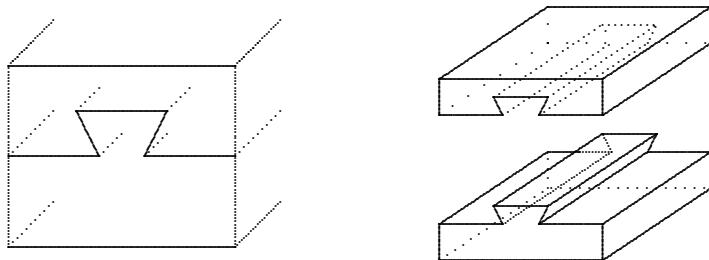
Here are two pictures showing *impossible* dovetails: an object made of two pieces of wood, with square footprint, and with identical view from all four sides: always, one sees the end of a dovetail.
