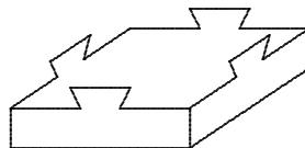
why should the dovetails be parallel to the sidewalls? There is a very simple solution (see the following pictures left and in the middle), using dovetails parallel to one diagonal (and then this diagonal direction is the sliding direction):
